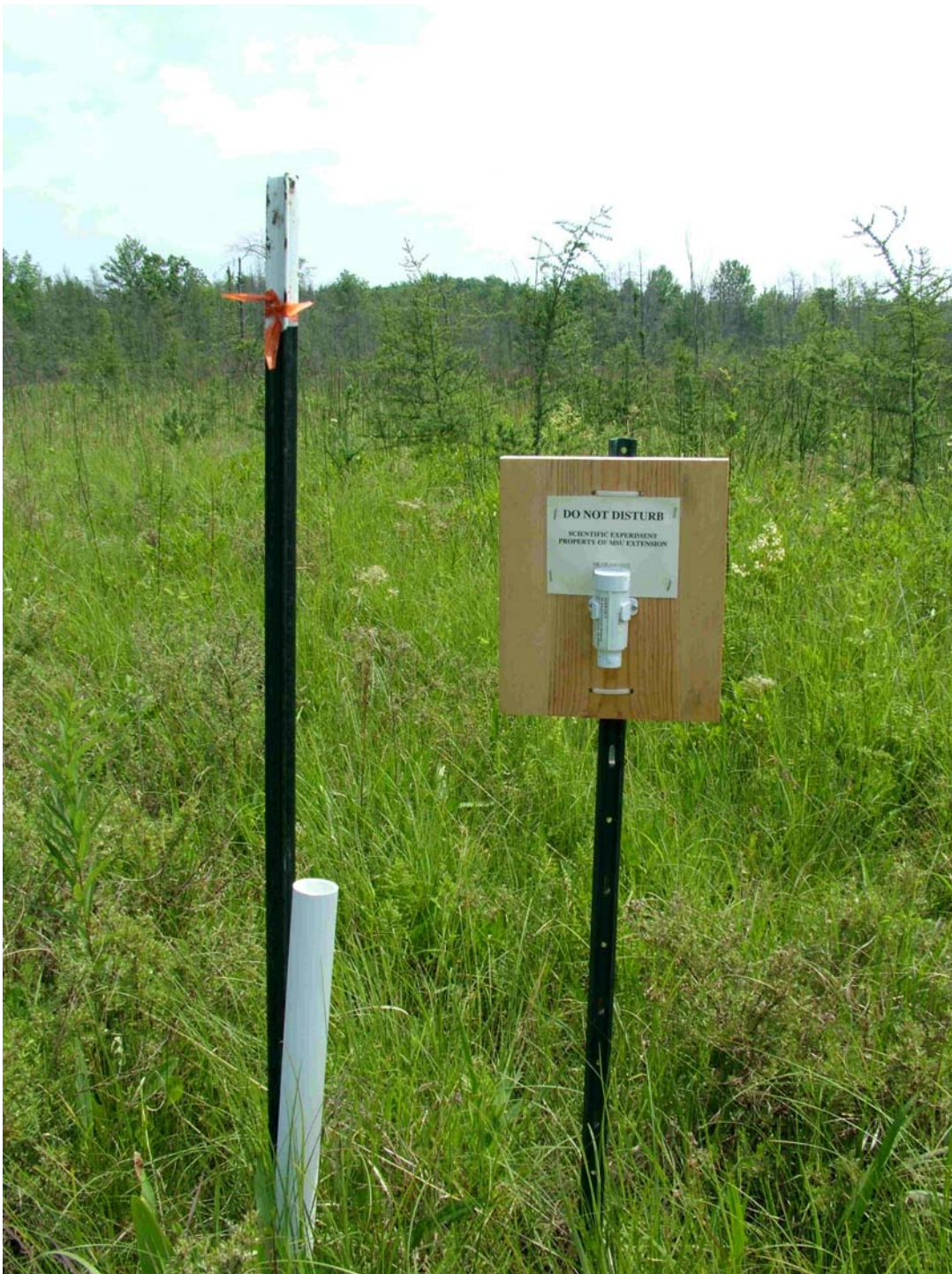
Figure 4. Hobo datalogger on metal fence post in fen. Data collected included hourly temperature and relative humidity readings.
